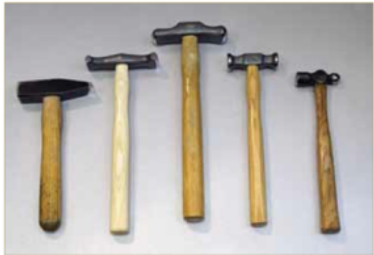
Basic shapes of steel hammers. From left to right: Forging, raising, forming, planishing and ball peen.
